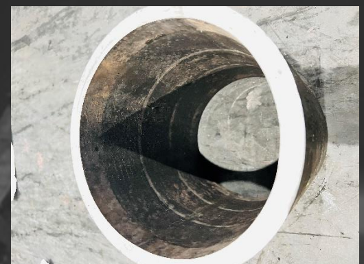
Rubber surface effect on casing inside surface
